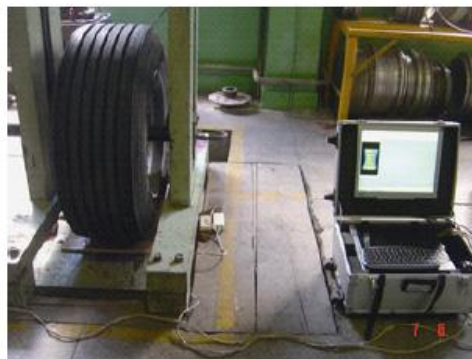
Figure 4.9.2 Sample tire, tire static loaded test machine and Tekscan [23].
