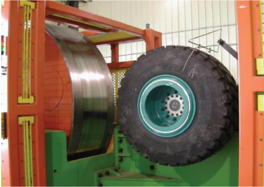
Figure 4.3.1 Drum testing machine [19].
