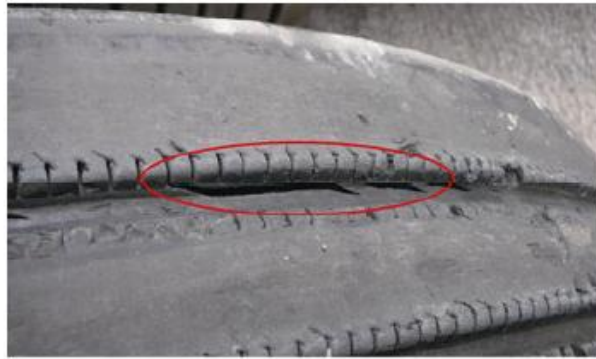
(a) T1 tire with cracks
