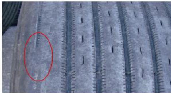
(b) T1 tire with shoulder wear seriously
