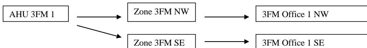
Figure 10: Sequence of assigning the spaces to AHUs
