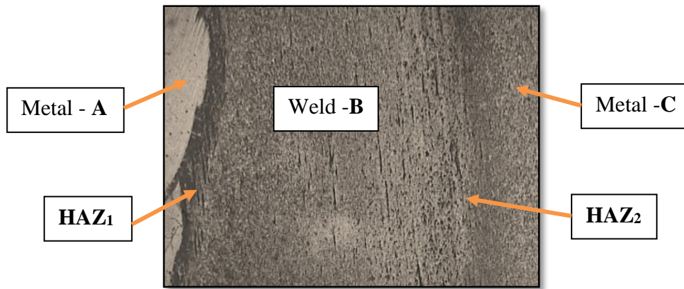
Figure 4.6 : Microstructure of all section of specimen -50X
