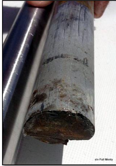
Figure 2.13 : Failed rudderstock of Catamaran hull sailing boat [37]
