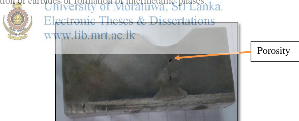
Figure 4.15 : Porosities on sample weld piece
