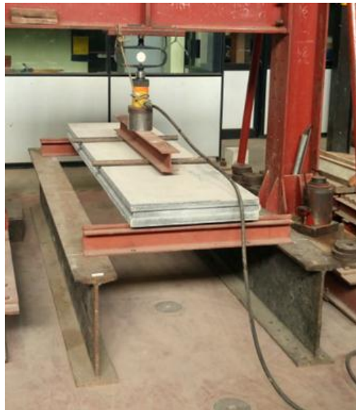
Figure 4.12: A Wall panel being tested for flexural strength
