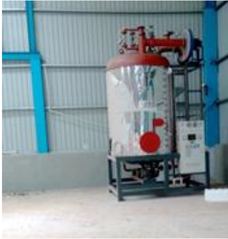
Figure 4.2: Steamer used to expand the polystyrene
