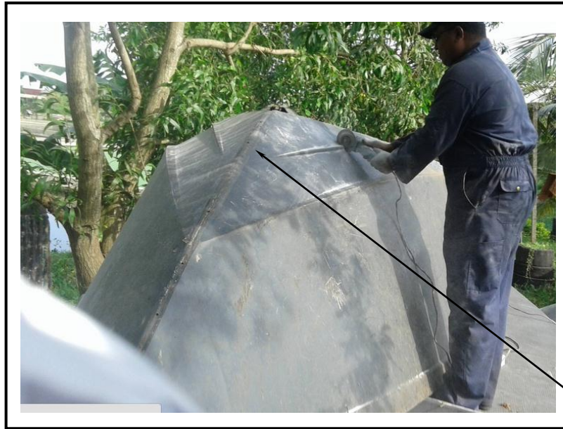
Figure 3.3: Specimens Extraction IPC keel area
