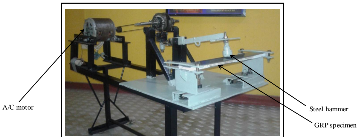
Figure 3.6: Tidal wave blow simulation machine
