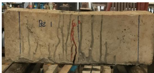
Figure 3.31: Failure pattern of B-C1
