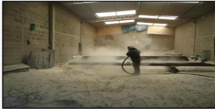
Figure 3.5: Sand blasting of beams
