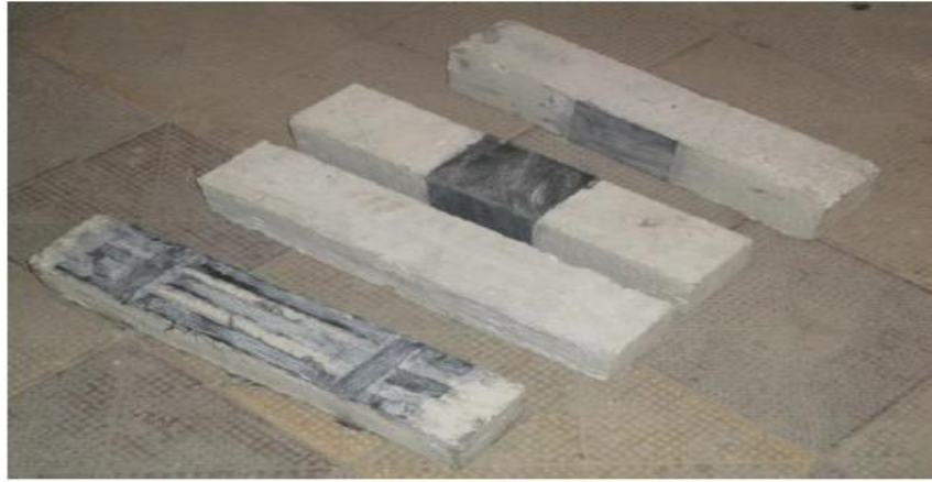
Figure 2.11: Different forms of CFRP wrapping on prisms
