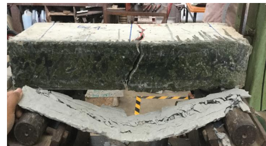
Figure 3.34: Failure pattern of C-PC2
