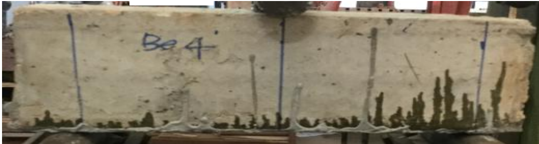
Figure 3.18: pasted CFRP laminate on primer coated beam sample
