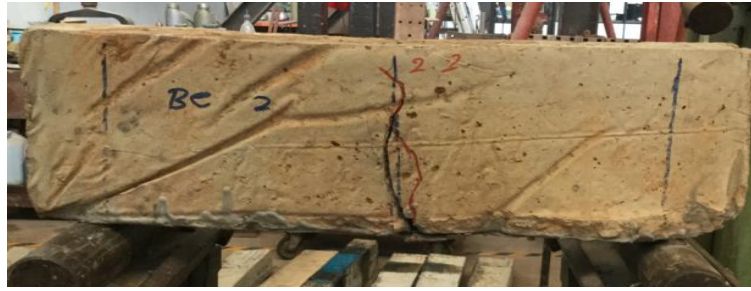
Figure 3.32: Failure pattern of B-C2
