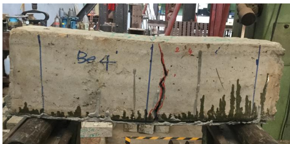
Figure 3.34: Failure pattern of C-PC2
