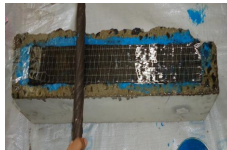
Figure 3.14: Attaching of CFRP and air removing
