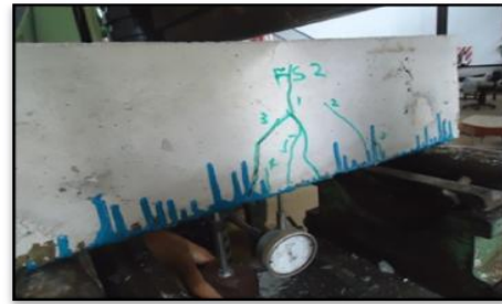
Figure 3.29: Failure pattern of A-E1 Figure 3.30: Failure pattern of A-E2
