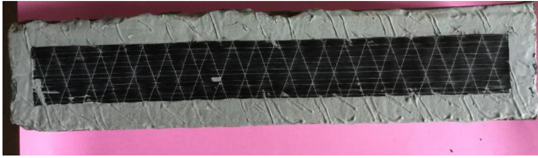
Figure 3.16: CFRP laminate pasted with cement grout
