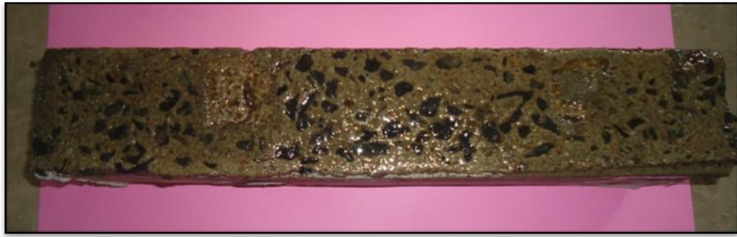
Figure 3.10: Primed surface of beam
