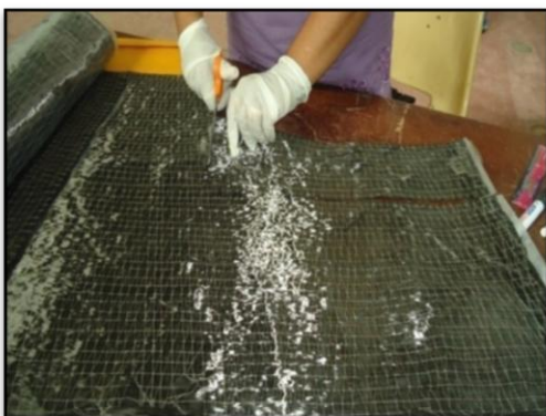
Figure 3.11: CFRP sample preparing
