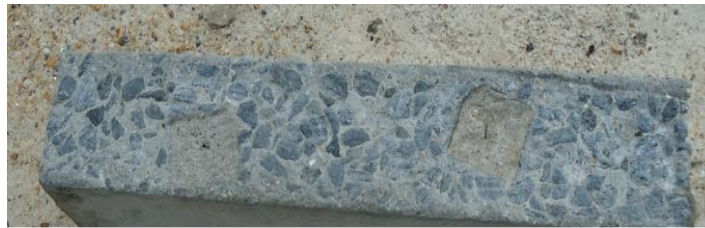
Figure 3.5: Sand blasting of beams
