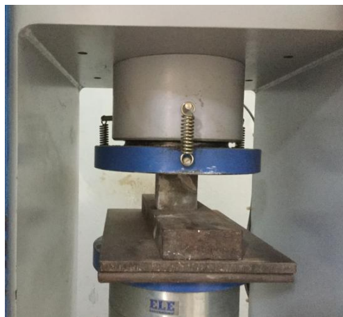
Figure 3.22: Cement grout testing
