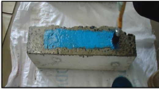
Figure 3.13: Application of saturant
