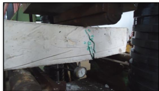
Figure 3.28: Failure pattern of C2
