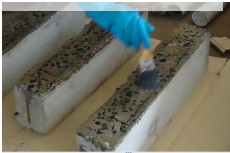
Figure 3.9: Application of Primer
