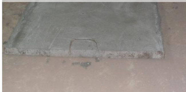
Figure 5.20: Trays Fofr Mixing Mortar and Concreting
