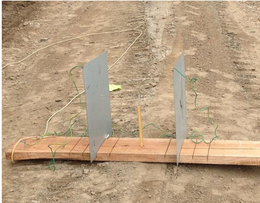
Figure 5.1: Investigating the behavior of detonator placed in an electric field in open air
