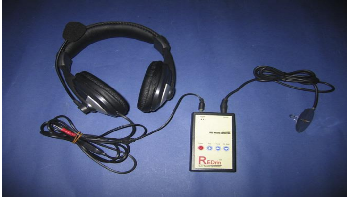
Figure 2.2 The acoustic device comprising the sensor, main unit and the set of headphones [6].
