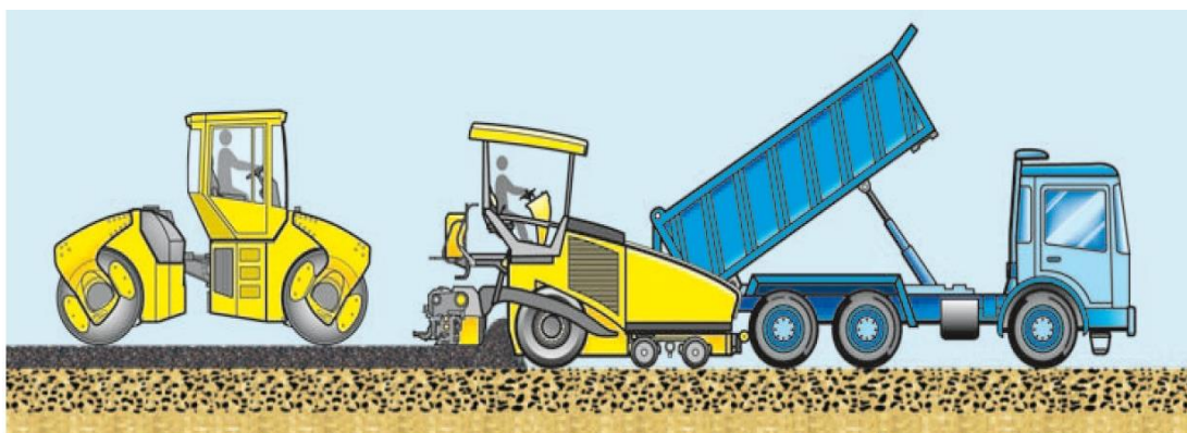
Figure 2-6: Initial compaction with the finisher
