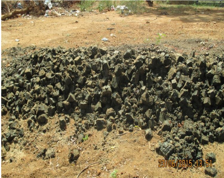
Figure 1.4: Dewatered and Disposed within the WTP Site or Open Dumping
