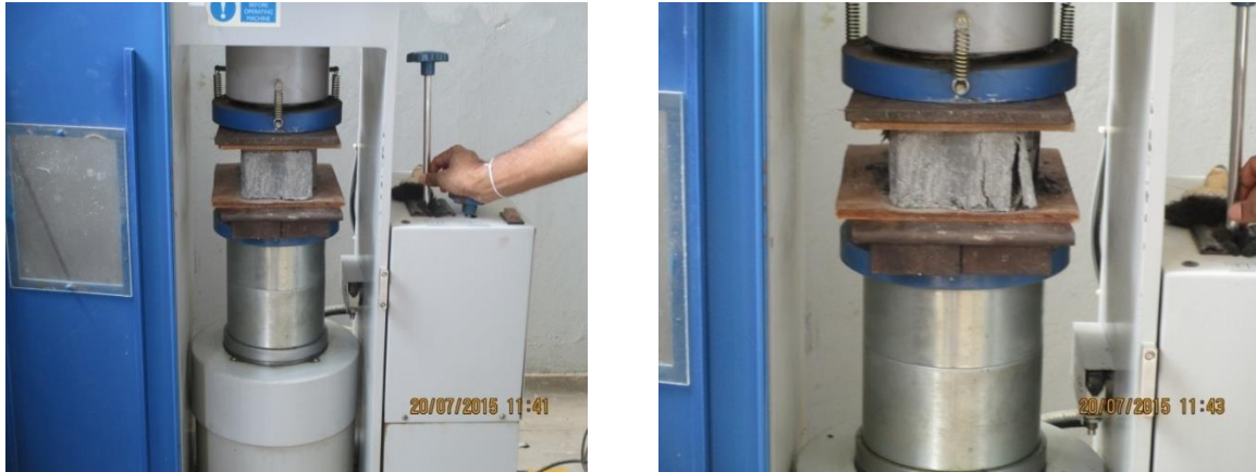
Figure 3.11: Compressive Strength Test on Concrete Paving Block
