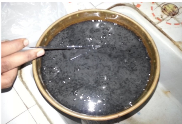
Figure 3.3 Cleaning of fly ash after activation
