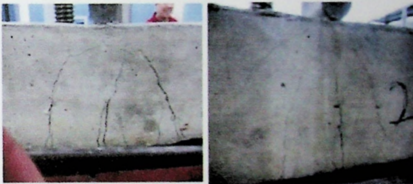
Concrete Beam with steel fiber Model 2 tested to destruction 28th day specimen
