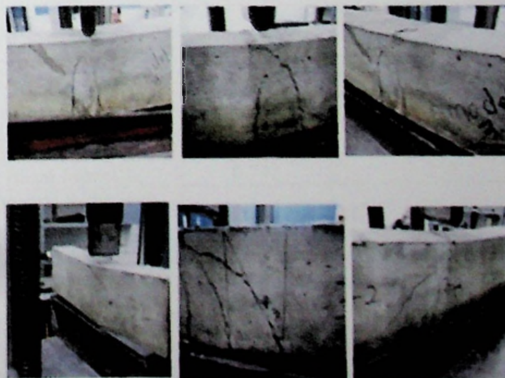
Concrete Beam with Steel fiber Model 3 tested to destruction 28th day specimen
