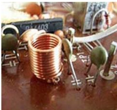
Figure 1.1: An air cored inductor
